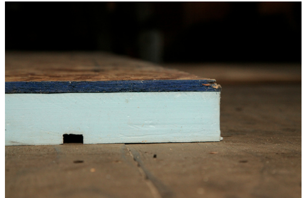
The factory-made foam and waferboard sandwich shown here is part of an insulated panel called Barricade. It's primarily sold for basement wall insulation, but also makes an excellent insulation option for warming up cold floors. Photo credit: Steve Maxwell
