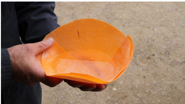
This cone of KERDI cloth holds water even though the seams aren't sealed. Installed underneath tile installations, it easily makes them 100% waterproof. Photo credit: Steve Maxwell
